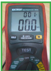
Fig. 6 - Valve Position Closed, Brown/Yellow, Continuity ◀ Correct
