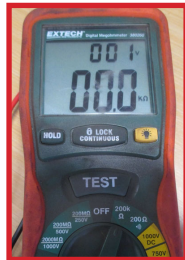
Fig. 3 - Valve Position Open, Brown/Yellow, No Continuity ◀ Correct
