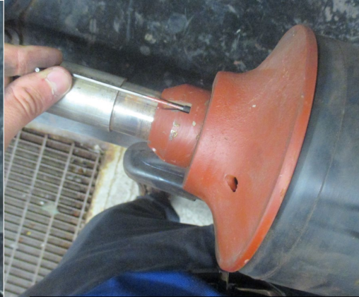
Fig 12. Reinstall drain nut set screw
