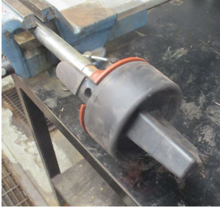
Fig 7. Secure lower stem in vice if possible
