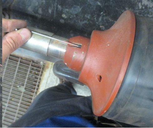
Fig 8. Loosen drain nut set screw with 5/64" or 2mm Allen key
