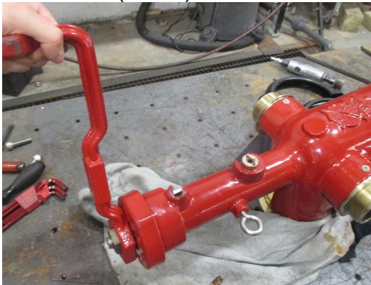
Fig 3. Unscrew upper barrel from the lower
