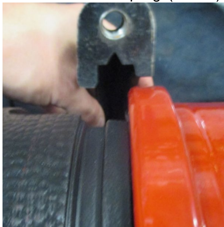
Fig 21. Note orientation of barrel coupling
