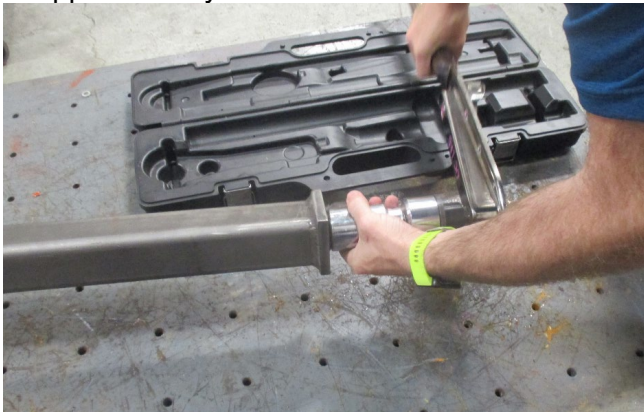
Fig 15. Slide seat removal wrench over breaker coupling
