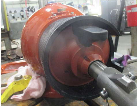
Fig 13. Lower main valve into hydrant, ensure main valve reaches bottom of elbow
