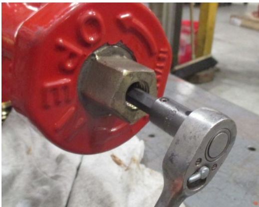
Fig 24. Tighten the op stop until a dead stop is felt
